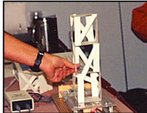
**Figure 3. A model building on a shake table.**
