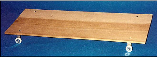
**Figure 2. A simple, horizontal motion shake table. Wheels are nylon cabinet or drawer wheels and are attached to the board with "L" brackets, machine screws and nuts.**
