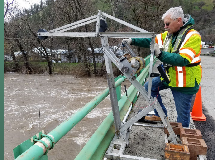
Upper Columbia Idaho Field Office Lead Technician, Keith Hein, measuring highflows on the S.F. Clearwater at Sites, ID - 13338500
