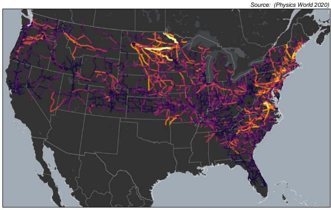
Figure 7-1. Voltages Induced by a 100-Year Super Geomagnetic Storm (Yellow 900 Volts to Dark Violet 10 Volts)
