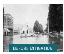
Problem: The City of Lewiston lies at the confluence of the Snake and Clearwater Rivers with USACE constructed dam, reservoir, and levees designed to protect downtown from a 100-year flood. The drainage system passes under a railroad and highway into the USACE system; however, high intensity rain events caused flooding behind the levees repeatedly damaging properties due to undersized stormwater drainage.
